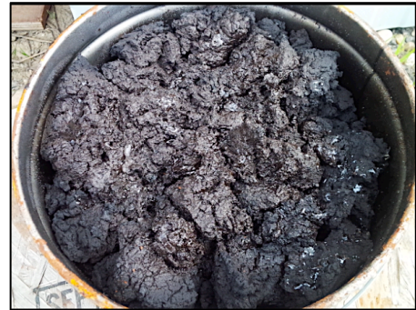
Fig 1: Oilfield Waste (Slop Solids) initially classified as hazardous waste material
